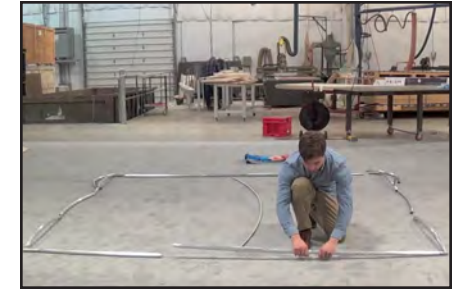
Insert the next tube until button lock engages.
