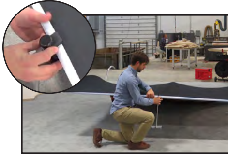
Attach lighting. Tighten clamp to secure lighting.
