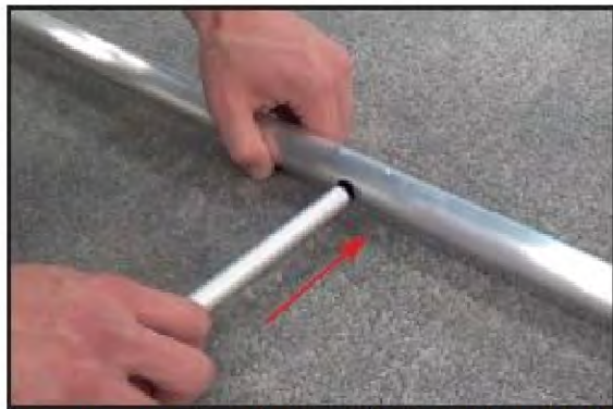
Insert support pole into TOP and BOTTOM of the frame.
