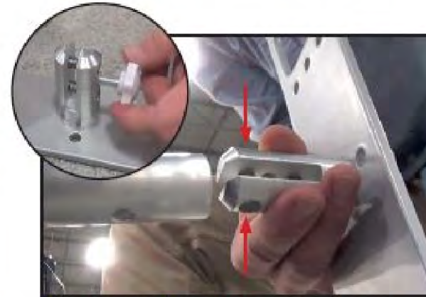
Attaching the feet, remove the thumb screw. Squeeze and insert. Repeat for other foot.
