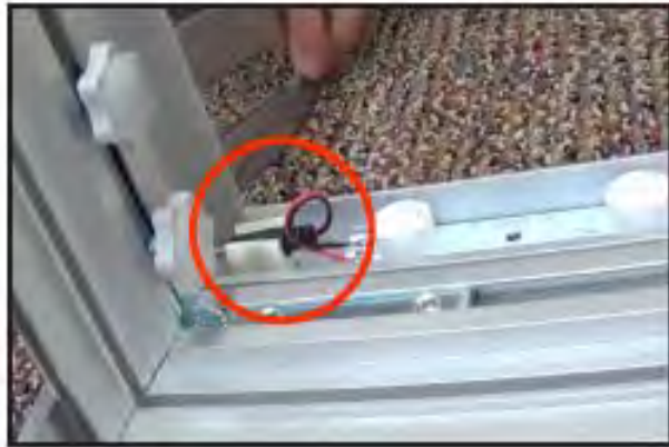
*Important* See that all LED connections are stowed in clips to prevent damage from mitre edges.
