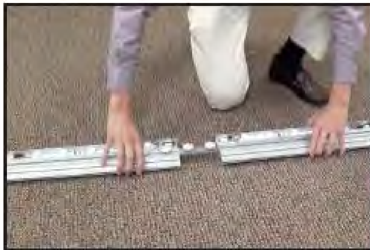
Connect bottom extrusions (Part 6 & 7) and tighten 2 thumb screws.
