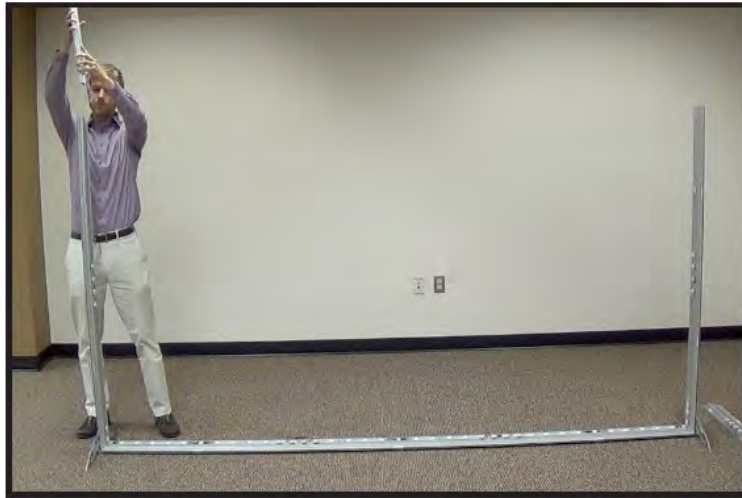
Connect upper left extrusion and tighten 2 thumb screws.
