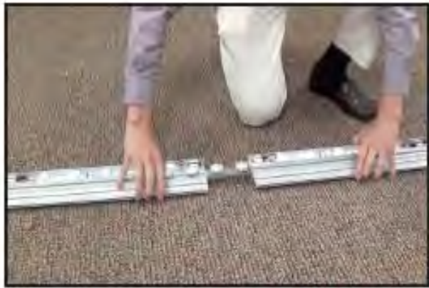
Connect middle extrusion and tighten 2 thumb screws.
