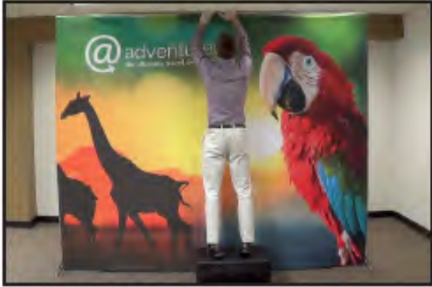
Insert SEG into top center channel.
