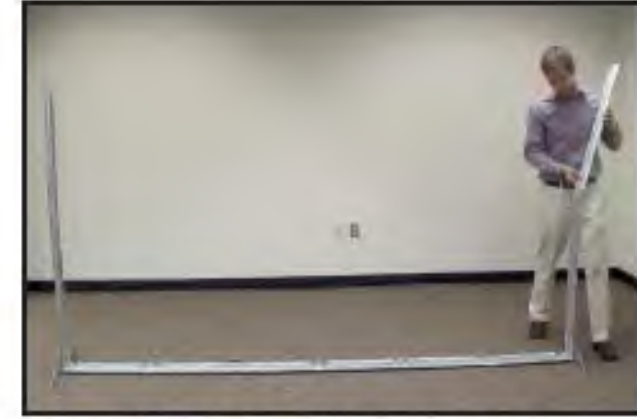
Connect middle right extrusion and tighten 2 thumb screws.
