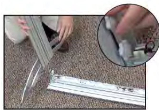
Connect extrusion assembly onto L-Bracket and tighten thumb screws.
