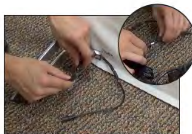
Connect the LED driver to the LED connector for the bottom row of lights and connect the other LED driver to the cord extension for the top row of lights.
