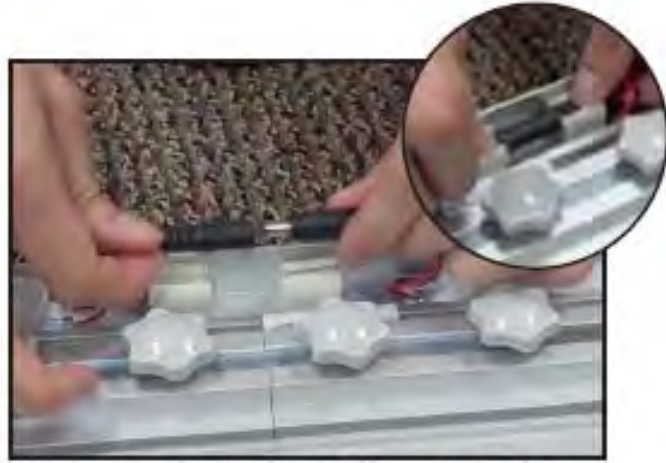
Remove LED connection from the clips. Connect the two ends and stow back into the clips
