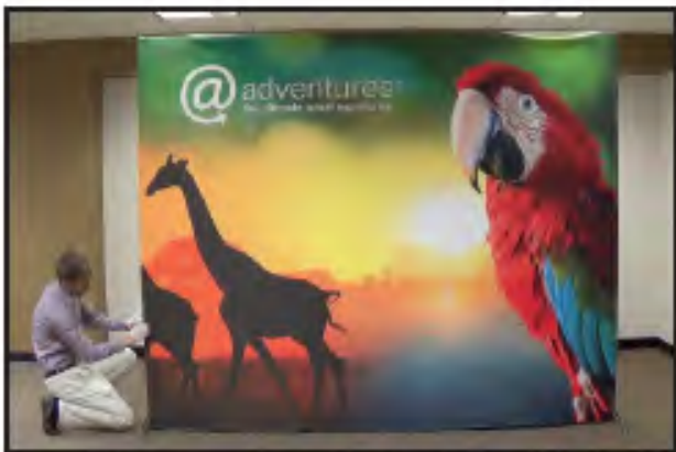
Press the remaining SEG into the channel along the left side.
