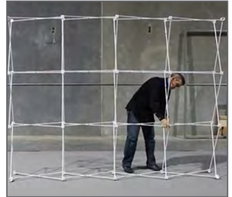
Lock the frame hubs together
