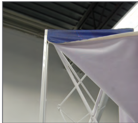
4. Install backlit front graphic, starting with endcaps
