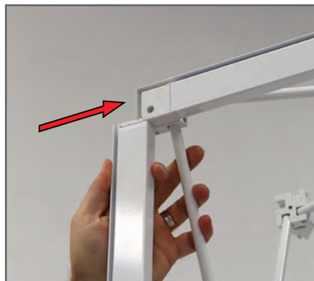
3. Hang the standard flat channel bars on the back of the frame
